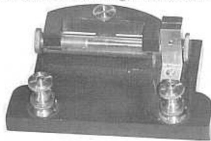
Fig. 7. The actual Mercury Detector used by Marconi at St. John's, now on display at the Science Museum, London (photo Bart Lee). Lane Upton functionally replicated Marconi's detector based in part on this photo.
