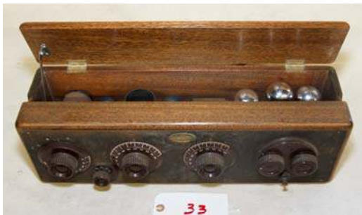
33. Atwater Kent / 33 1927; TRF; Broadcast band; has tubes including two Arcturus 201a tubes.
