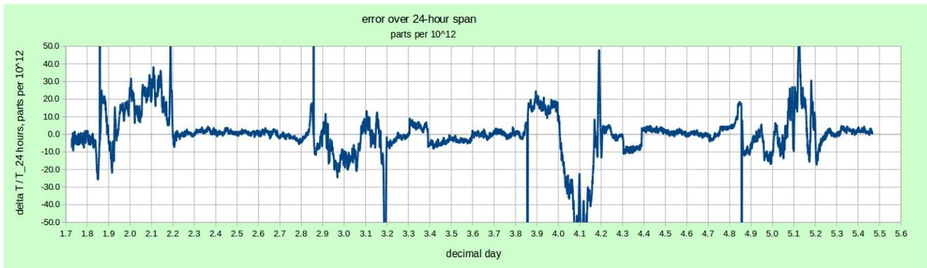
Between day 2.25 and 2.8, the differential time difference is less than  $2 \times 10^{-12}$ , with an rms spread of  $1.3 \times 10^{-12}$ .
