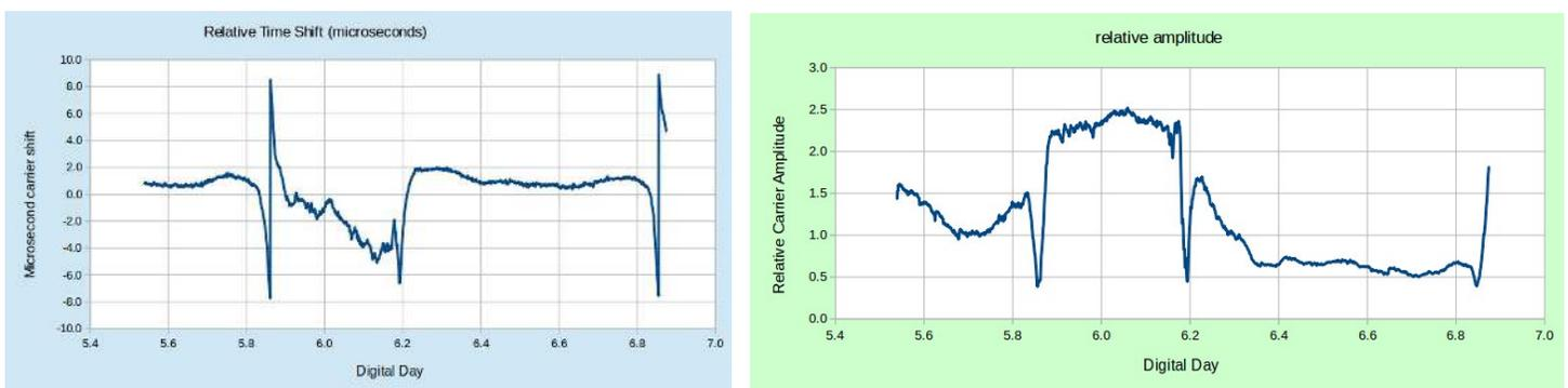
The time variation of the carrier phase from day 5.5 is shown on the left, and the relative amplitude on the right. Since the WWVB signal is amplitude modulated with a 17 dB modulation depth, to measure the average carrier level, the signal strength was sampled 20 times a second, and then integrated over 60 seconds for each data point.
