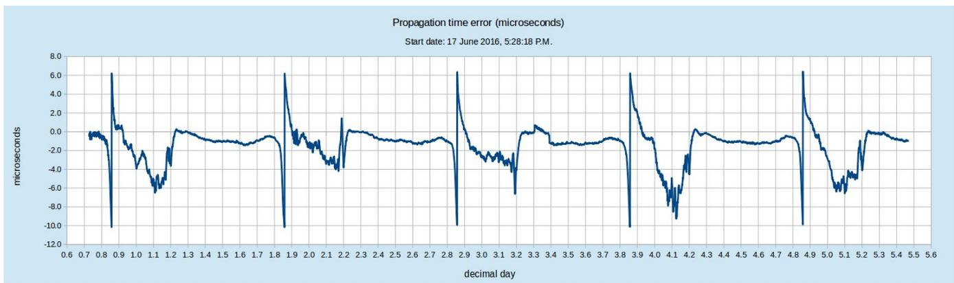
The abscissa is in units of days (N). The plot starts at day 0.7322 or 17 June 2016 05:28:18 P.M. (N = 0, 1, etc.) is midnight, (N+0.5) is noon. The ordinate is the time shift in microseconds of the WWVB carrier relative to the GPS reference. The ordinate of the plot is modulo 16.667 microseconds, so larger excursions are folded on the plot. (The plot looks almost like an electrocardiogram.)
