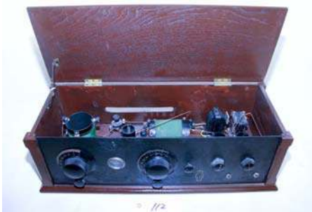
112. Browning-Drake / model? 1920's; Regenerative; kit assembled; no tubes
