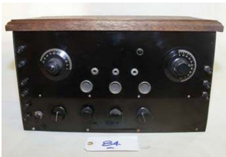
84. Homebrew / model? 1920's; 3-tube Regenerative; no tubes
