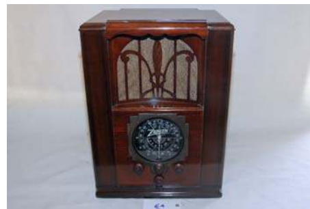
64. Zenith / 6V27 1936; Battery farm set converted to work on 120vac; Restored
