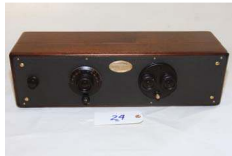
24. Atwater Kent / 49 1928; TRF; no tubes
