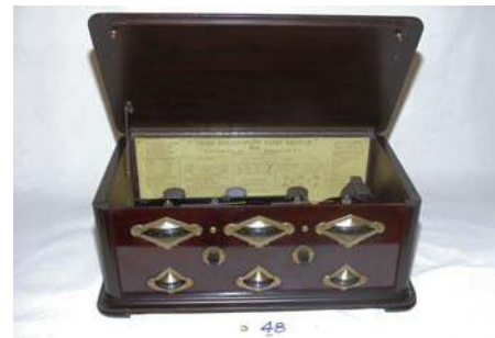
48. Grebe / MU1 Syncrophase 1925; TRF; with chain; no tubes
