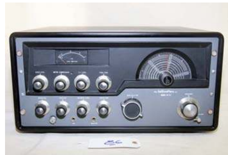
86. Hallicrafters / HT-32 1958/59; Transmitter; SSB/AM/CW; 80-10 meters
