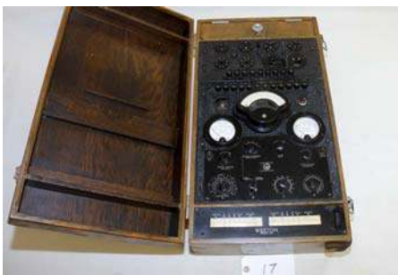
17. Weston / 788 1943ca (WW II); Tube tester/analyzer; built for the US Navy
