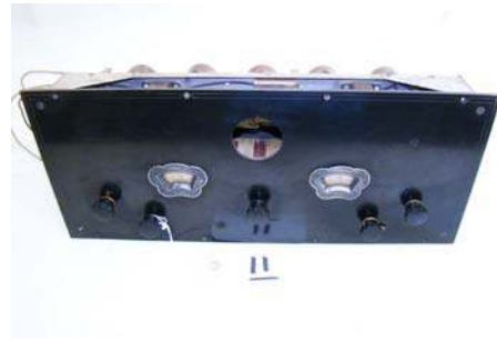
11. Kennedy / 30 1925; TRF; AM Broadcast; panel with chassis only, no cabinet
