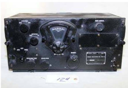
124. US Army Signal Corps / BC-348-Q WWII era; 5 bands covering 1.5 - 18.0 MHz;
