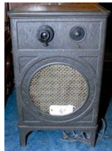
61. Atwater Kent / 52 1928; TRF; AM Broadcast; Unique all-metal small console cabinet
