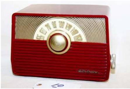
10. RCA Victor / 1X56 1952; AM Broadcast; working, restored
