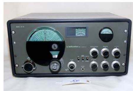
56. Hallicrafters / SX-42 1946-1948; AM-CW-FM Receiver; Fully covers 0.540 -110MHz in 5 bands (80,40,20,10,6 meters)
