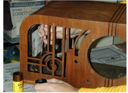
Figure 12: Coloring the edge of the speaker grill opening.
