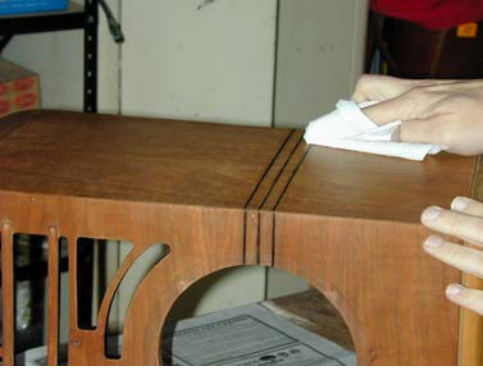
Figure 13: Cleaning slop-over from groove edges.
