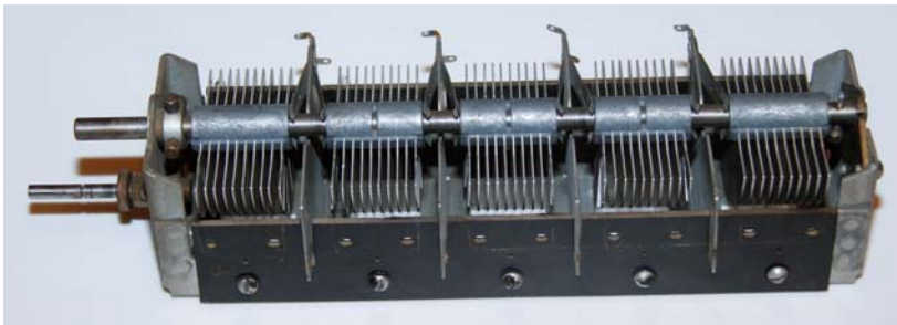
Figure 2: The five-section tuning capacitor showing the rotor assembly and frame; the stator assemblies have been removed.
