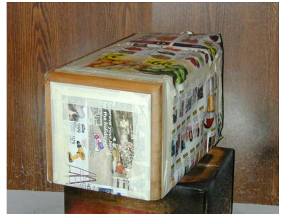
Figure 14: Mask off the cabinet to only expose the trim area for coloring.
