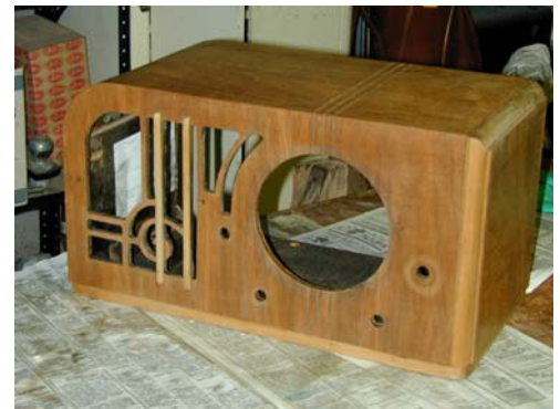
Figure 11: The stripped cabinet.
