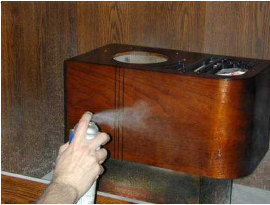
Figure 17: Spraying the clear coat.
