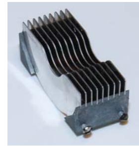
Figure 3: A stator assembly showing the cast pot metal holding the blades.
