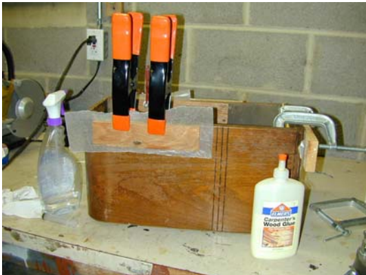
Figure 6: Clamping the loose veneer.
