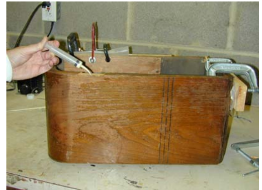
Figure 5: Using a glue syringe.
