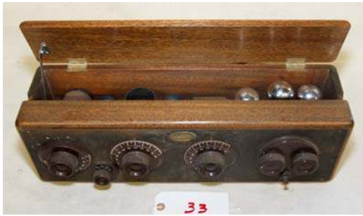
33. Atwater Kent / 33 1927; TRF; Broadcast band; has tubes
