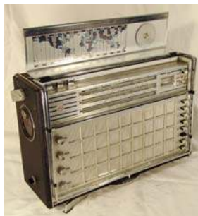
85. Philips Norelco / L6X35T/54 1967; BC/LW/SW; solid state
