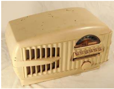
73. Belmont / 6D121 1847; Broadcast band; electronically restored
