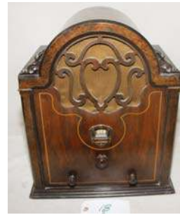
18. Howard / SG-B 1930; TRF; Broadcast band
