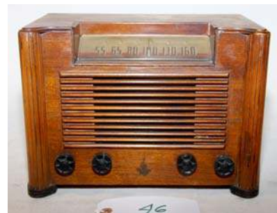
46. Emerson / 442? 1940/41; Broadcast band; electronically restored; has audio input
