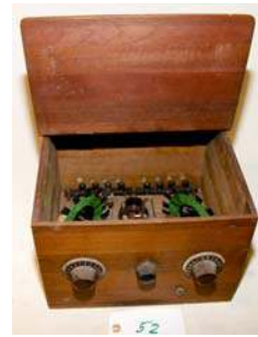
52. Homebrew / . Early-mid 1920s; one tube receiver
