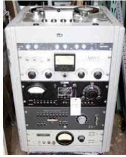
97. Ampex / 350 reel-reel tape rack Includes: GR1932A Distortion indicator, GR1301A osc, Daven audio panel; was in KQED
