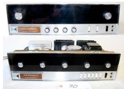
70. Heathkit / AJ-15/AA-15 1968; Stereo system with tuner (AF-15) and 100W amplifier (AA-15); both working
