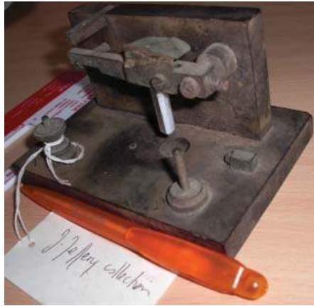
Figure 6. This incomplete device was found amidst the artifacts preserved by Porthcurno technician John Jeffery, and examined in 2010 at Porthcurno Archivist Alan Renton's request. Note the filed-off thermometer glass, the lever arm that can move it up and down, and the circular trace beneath it. The base measures 90 mm deep (3.5 inches). Photo by Bart Lee.
