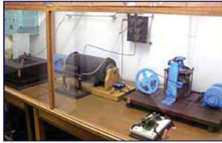
Figure 23. A display of the Type 36 wireless telegraphy system circa 1905, on display aboard the memorial battleship Mikasa in Japan. The coherer receiver is on the far left. In the center is a 30 cm (12 inch) inductance coil and spark gap in front of it. The antenna transmit -receive switch is at the top center above it. The motor and belted wheel device on the right may be a motor generator to power the spark coil primary. The device in front of it may be a keying relay. Image from Rear Admiral Kazuo Itoh, The Battle of Tashima Was Real Network Centric Warfare , [note 4].
