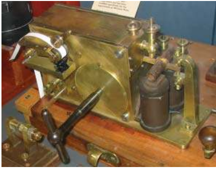
Figure 2. The modified cable inker for recording signals on paper tape, likely the one used by Maskelyne to record Marconi wireless transmissions. It was found amidst the artifacts preserved by Porthcurno technician John Jeffery. It is now on display at the Porthcurno Museum. Photo by John E. Packer.
