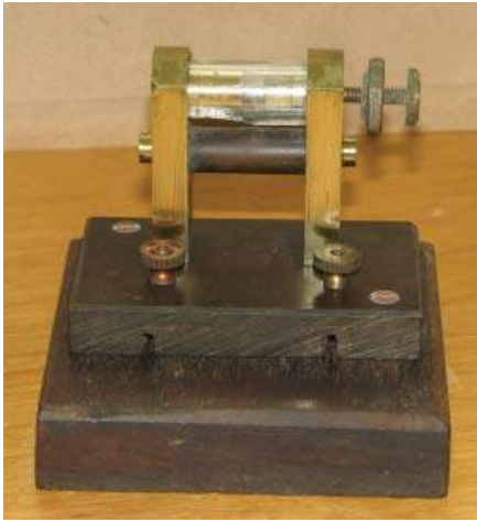
Figure 5. A coherer that was found amidst the artifacts preserved by Porthcurno technician John Jeffery. It is now on display at the Porthcurno Museum. Photo by John E. Packer. Nevil Maskelyne patented a coherer of a different (compression) design that he called a "conjuncture." According to Packer's Spies at Wireless Point [note 2] conjunctures from Maskelyne were in use there in 1903 with variable results, along with some other but unreliable Hozier-Brown receiving equipment (page 16).
