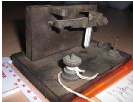
Figure 7. A closer view of the incomplete device preserved by Porthcurno technician John Jeffery, as examined in 2010. The filed-to-a-point thermometer glass has an uncorroded, perhaps platinum, wire threaded down its center. Photo by Bart Lee.
