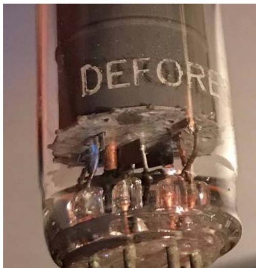
The CHRS tube is a 5AQ5 TV and HiFi era tube, so maybe it isn't the actual World's First Tube, but a late descendent of De Forest's Audion of 1906. The 5AQ5 like the 6AQ5 sits in a seven-pin "miniature" glass envelope. Primarily, the 5[&6]AQ5 functioned as an audio beam power amplifier. The box claims "Hi-Fi Quality performance" (TV sets also used them).
